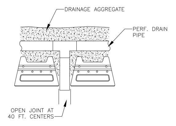
DRAIN DETAIL SCALE: 1"=1'
